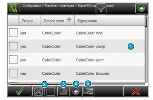
**Create new assignment:** Creates a new list entry of a signal I/O assignment **4**. A screen is shown, where the signals can be assigned to the built in hardware interfaces accessible on the rear of the machine.
