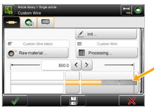
The article can be programmed directly as "User defined application". However, switching to "Userdefined application" after a predefined application has been previously programmed, all settings of the predefined application are adopted.
