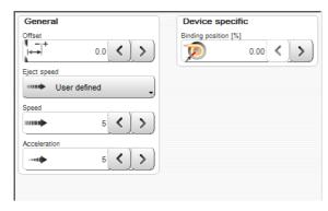
**Eject speed:** With the setting "Feed speed" the article is ejected with the speed defined under
