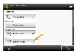
The "Library mode" provides additionally the application type called "User defined". This way also multi-step stripping can be performed.
