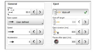
**Eject speed:** With the setting "Feed speed" the article is ejected with the speed defined under "Processing - feed". Optionally a user defined combination of "Speed" and "Acceleration" can be set for the ejection.
