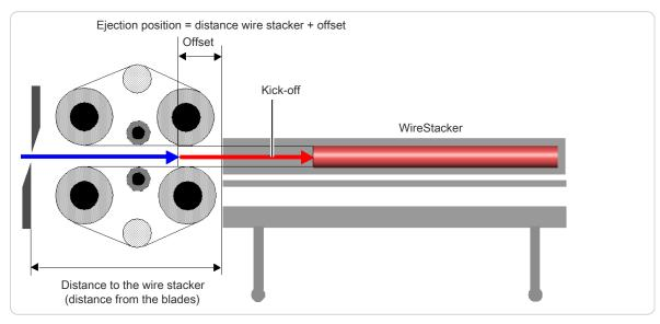
Fig. 29: Ejection with "Kick off" activated
