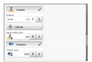
**Feedback:** Deactivated = The signal is transferred according to the signal duration, after the waiting time the *MegaStrip 9680* continues with the production.
