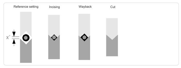
Fig. 10: Position of blades while feeding
