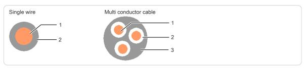
Fig. 18: Layer sectioning
