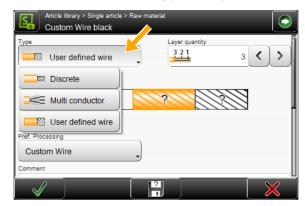
**Discrete:** The outer- and inner diameter of a single wire can be entered separately.
