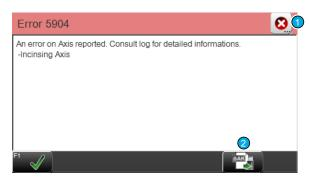
With the "Data Backup" button 2 all log files stored on the machine can be saved to a USB data storage medium. These logs are for the *Schleuniger* support and serve for the exact analysis of hardware problems.
