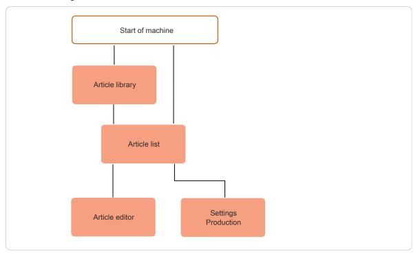
Fig. 23: Principle, "Article list mode"
