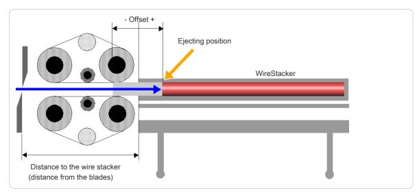
Fig. 28: Ejecting with offset
