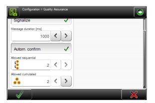
As soon as one of the two counters is reached and the defective piece has been rejected, the machine stops and error message 5955 appears with the following informations:
