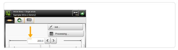
If the correction mode is on, the user opens directly the numeric touch-keyboard by touching [ENTER CORRECTION VALUE] where the effective measured length can be entered.
