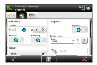
Rejected pieces (including those detected by SmartDetect) can be declared good after manual verification, i.e. the rejected piece can be manually ignored. This option is only offered if the "Ignore" setting is activated in the "Monitoring" menu in the configuration.
