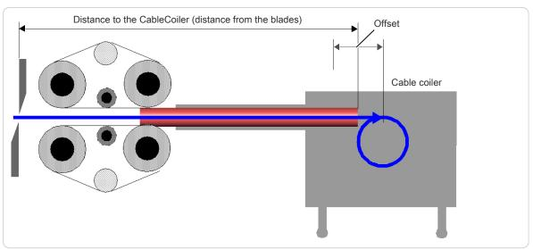
Fig. 30: Ejecting position cable coiler
