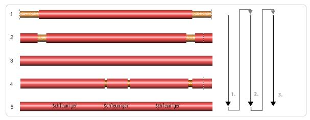
**Single article first:** The *MegaStrip 9680* produces the "Total" of each article fully (Quantity of "List passes" x "Article quantity"), before proceeding to the next article. This mode is especially recommended when different Raw materials are used. Less waste is produced.
