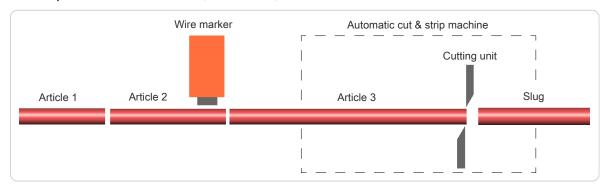
Fig. 5: Processing without slug
