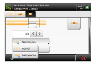
2. In the Processing editor, the autonomous element is marked with a white "i" on a blue background.
