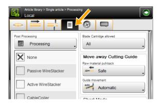
**Local:** If for a designated article a defined post processing device is used, it can be selected in the local Processing. This type of Processing is recommended if a designated article has to be produced differently from the programmed single article in the list.
