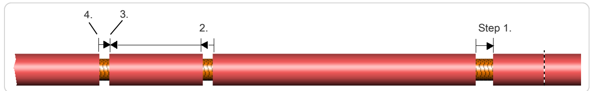
Fig. 13: For example, pull-off in several steps
