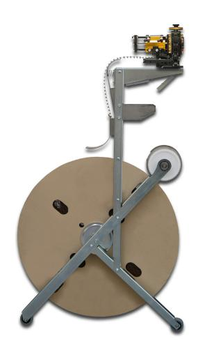
**ToolingShuttle 30**Mobile Quick-Change Unit for CrimpCenter Series
